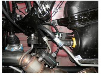
**Step 6.** Re-connect the wiring harness plugs to the Valve motors.
