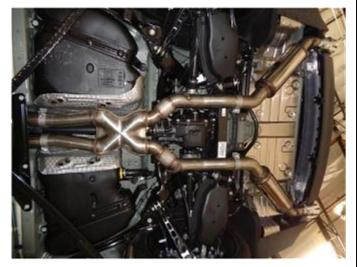
**Step 5.** Install the Muffler Assemblies to the X-Pipe Assembly with the supplied 2.75" clamps and engage the welded hangers to the rubber insulators. Leave all clamps loose for final adjustment of the system.
